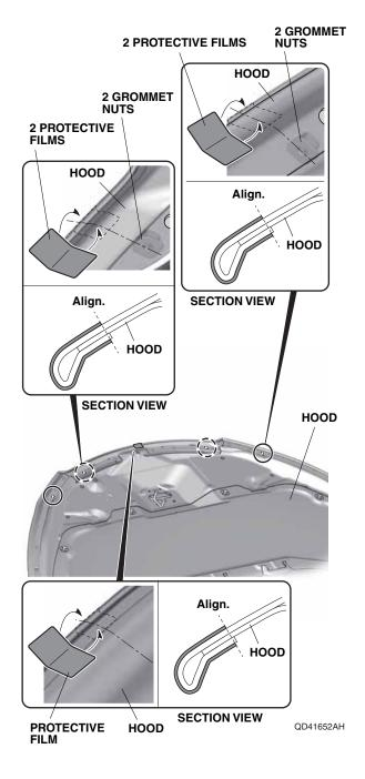
4. Slide the two brackets B and the two brackets C between the hood and the rubber molding as shown, and align them with the holes in the grommet nuts. Loosely install a truss screw through each bracket.
