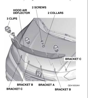
7. Make sure the edge of the molding on the hood air deflector unfolds.
