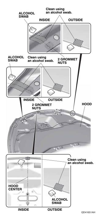
3. Remove the adhesive backings from the five protective films, and attach them to the front of the hood as shown.
