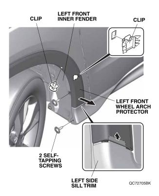
Remove two self-tapping screws and one clip. Pull out the left front wheel arch protector to release the clip.
