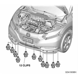
Remove four clips and two self-tapping screws on each side.
