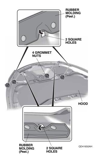
Using an alcohol swab, thoroughly clean the hood where the protective films will attach.
