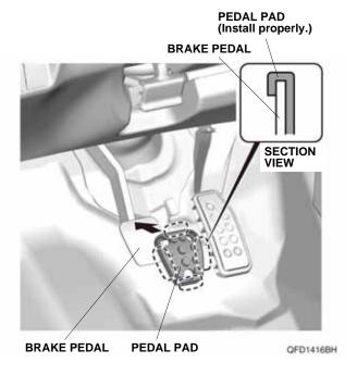
16. Using a white marker, mark the brake pedal as shown.
