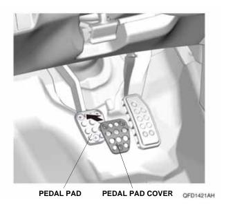
21. Using the hand riveter, install the pedal pad cover on the brake pedal with three rivets B as shown.
