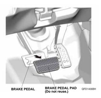
Install the new brake pedal pad onto the brake pedal.
