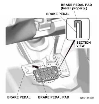
8. Using a white marker, mark the brake pedal as shown.
