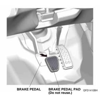
Install the pedal pad onto the brake pedal.
