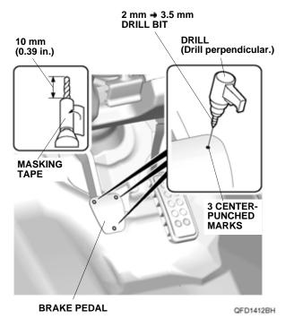
Install the pedal pad onto the brake pedal.
