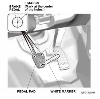
17. Remove the pedal pad. Using a center punch, punch the centers of the three marks. If using an automatic center punch, set it to the minimum setting.
