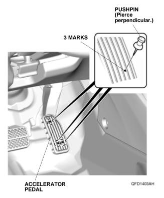
4. While wearing eye protection, drill the accelerator pedal at the three pierced marks using a 2 mm drill bit first, then finish using a 3.5 mm drill bit.
