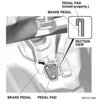
20. Loosely install the pedal pad cover on the pedal pad.
