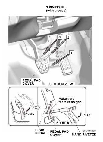
22. Repeat steps 14 through 21 to install the pedal pad and pedal pad cover on the clutch pedal.
