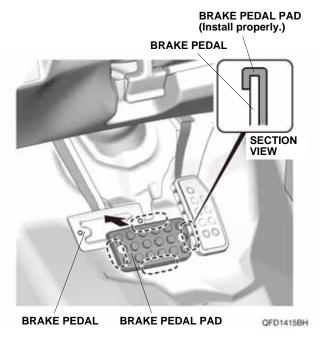
12. Loosely install the brake pedal pad cover on the brake pedal pad.
