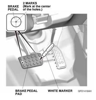
Remove the brake pedal pad. Using a center punch, punch the centers of the two marks. If using an automatic center punch, set it to the minimum setting.
