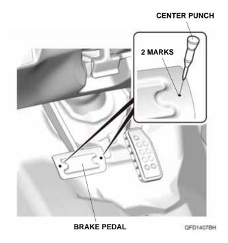
10. While wearing eye protection, drill the brake pedal at the two center-punched marks using a 2 mm drill bit first, then finish using a 3.5 mm drill bit.
