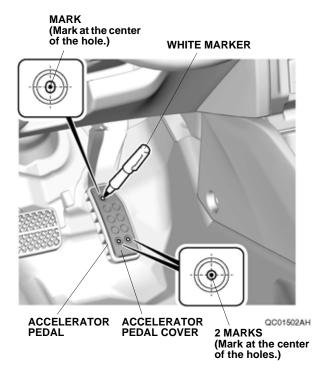
2. Using a white marker, mark the accelerator pedal as shown.
