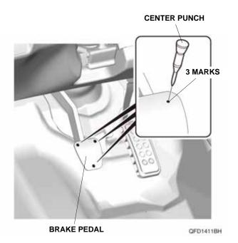
18. While wearing eye protection, drill the brake pedal at the three center-punched marks using a 2 mm drill bit first, then finish using a 3.5 mm drill bit.
