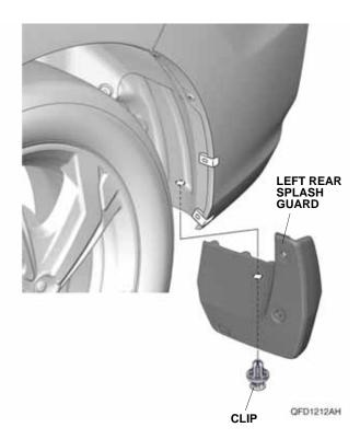
17. Secure the left rear splash guard with two 5 x 20 mm self-tapping screws as shown.
