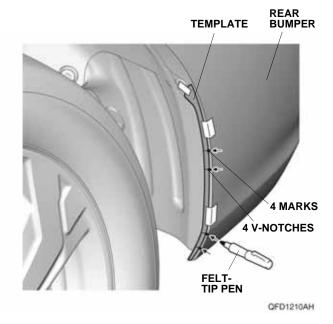
14. Carefully remove the template. Do not damage the template; it is also used to mark the right side of the rear bumper.
