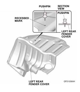
8. While wearing eye protection, drill the left rear fender cover at the pierced mark using a 3 mm drill bit first, then a 6 mm drill bit, an 8 mm drill bit, and finish using a 10 mm drill bit.
