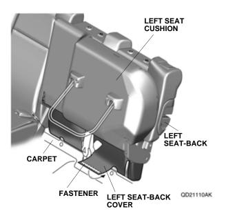
Lower the left seat cushion, and fold the left seat-back fully forward. Pull the seat-back cover tight, and secure it to the left seat-back with five fasteners.
