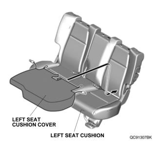
9. Install the two seat belt buckles into the loops.
