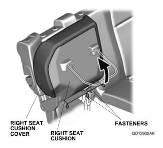
20. Secure the right seat cushion cover to the right seat cushion with two hooks and two loops, and lower the right seat cushion.
