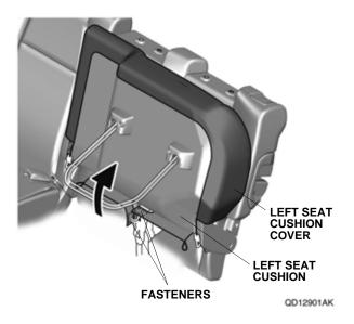
11. Secure the left seat cushion cover to the left seat cushion with the two hooks and two loops, and lower the left seat cushion.
