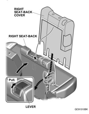
13. Lift up the right seat cushion. Secure the fastener on the right seat-back cover as shown.
