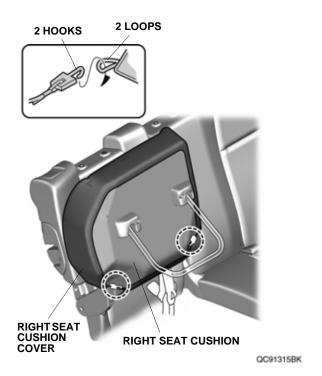
21. Install the head restraints on the seat-backs.
