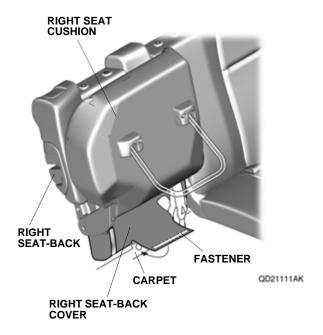
Lower the right seat cushion, and fold the right seat-back fully forward. Pull the seat-back cover tight, and secure it to the right seat-back with four fasteners.
