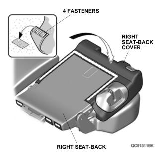
15. Lift the right seat-back. Tuck the right seat-back cover under each head restraint guide as shown. NOTE: Make sure that the lower anchor holes are not hidden by the cover.
