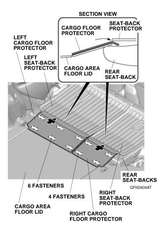
Check the protectors by moving the rear seat-backs back and forth.
