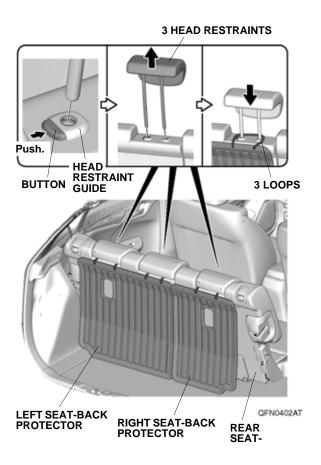
2. Fold down the rear seat-backs. Position the left and right seat-back protectors on the rear seat-backs. Secure the left and right seat-back protectors to the rear seat-backs with the 10 fasteners.
