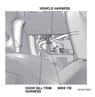
20. Route the door sill trim harness as shown. Align the green tape on the door sill trim harness with the vehicle wire tie, and secure the door sill trim harness to the vehicle harness with one wire tie.
