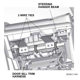
22. Route the door sill trim harness as shown. Then secure it to the vehicle harness with two wire ties.
