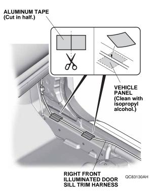
49. Using scissors, cut the aluminum tape in half.
