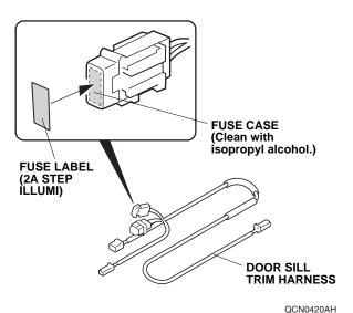
11. Attach the fuse label to the door sill trim harness fuse case.
