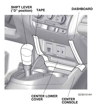
Remove the center lower cover, and unplug the vehicle connectors.
