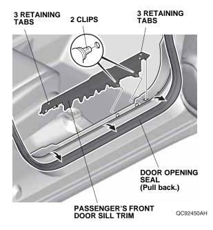
5. Pull back the door opening seal, and remove the passenger's kick panel.
