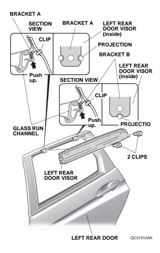
16. Adjust the left rear door visor to the position as shown.
