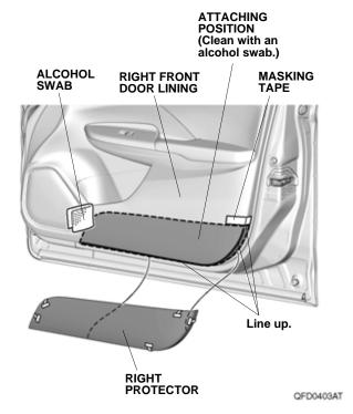
5. While applying light pressure against the right protector, carefully remove the taped adhesive backings.
