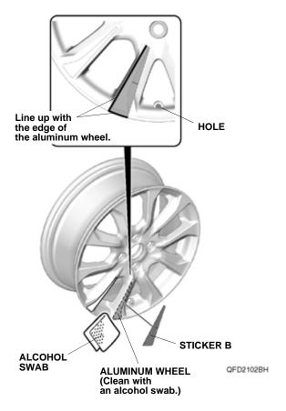
8. Line up sticker B with the edge of the aluminum wheel, and attach it as shown.
