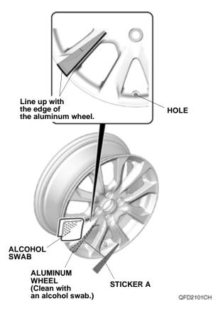
3. Line up sticker A with the edge of the aluminum wheel, and attach it as shown.
