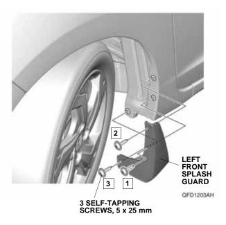
Turn the steering wheel fully clockwise, and repeat steps 2 and 3 to install the right front splash guard on the right side of the vehicle.
