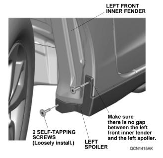
6. Loosely install the left spoiler with masking tape.
