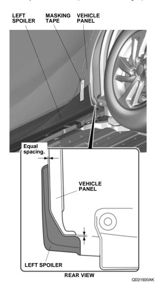
7. Using a felt-tip pen, mark the vehicle panel as shown.
