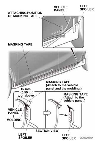
9. Remove the left spoiler while leaving the masking tape on the vehicle panel.
