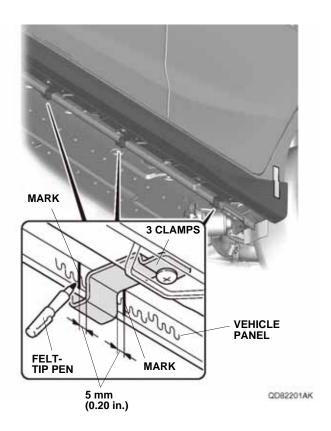
8. Attach the masking tape to the vehicle panel as shown.
