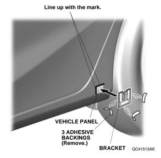
17. Line up the bracket with the mark, and attach it to the vehicle panel as shown. Press and hold the bracket firmly against the vehicle for 30 seconds.
