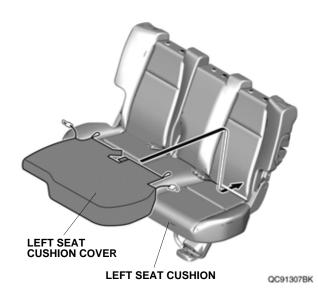
9. Install the two seat belt buckles into the loops.
