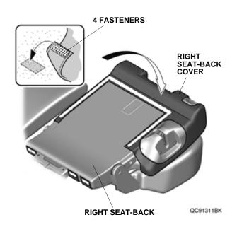
15. Lift the right seat-back. Tuck the right seat-back cover under each head restraint guide as shown. NOTE: Make sure that the lower anchor holes are not hidden by the cover.
