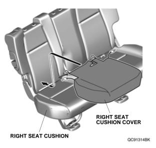
18. Install the two seat belt buckles into the loops.
