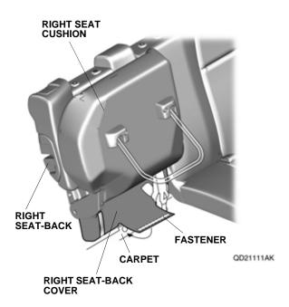
14. Lower the right seat cushion, and fold the right seat-back fully forward. Pull the seat-back cover tight, and secure it to the right seat-back with four fasteners.
