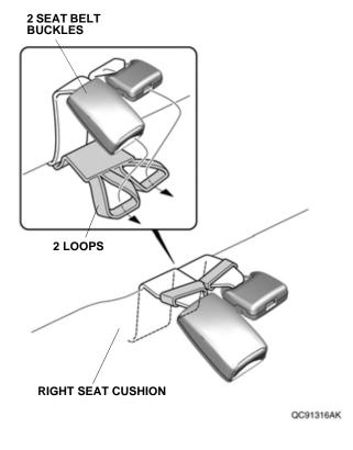
19. Lift up the right seat cushion. Secure the fasteners on the right seat cushion cover as shown.
