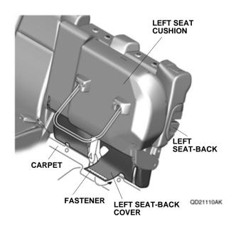
5. Lower the left seat cushion, and fold the left seat-back fully forward. Pull the seat-back cover tight, and secure it to the left seat-back with five fasteners.
