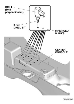
35. While wearing eye protection, enlarge the three holes to 5 mm.
