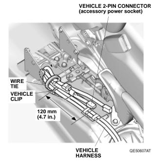
28. Plug the vehicle 12-pin connector into the center console sub cord 12-pin connector.
