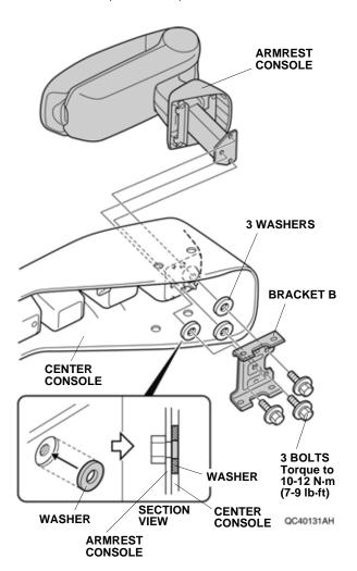
70. Plug in the vehicle connectors, and install the center console with one screw, four bolts, and three clips.
