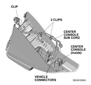
12. Remove the driver's and passenger's seat heater switches.
