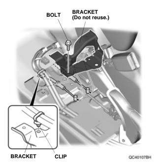
22. Cut off the clip from the vehicle wire tie. Go to step 24.
