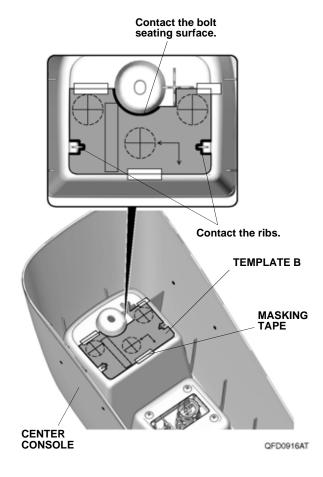
65. Using a pushpin, pierce the center of the three marks on template B.
