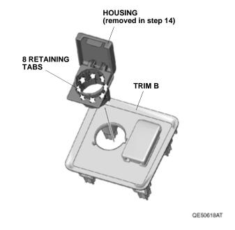
52. Install the accessory power socket in the housing.
