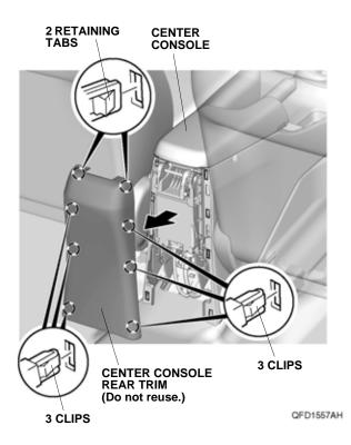
8. Remove the center console, and unplug the vehicle connectors.
