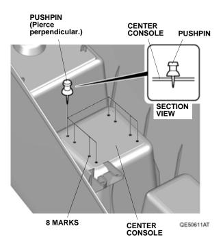
44. While wearing eye protection, drill the eight pierced marks with a 3 mm drill bit, then finish with a 5.5 mm drill bit.
