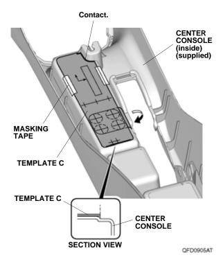
31. Using a pushpin, pierce the center of the nine marks on template C.
