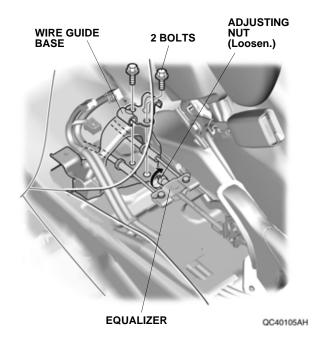
20. Disconnect the parking brake cables from the equalizer.
