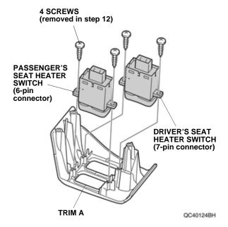
40. Install trim A on the center console with three self-tapping screws. Go to step 42.
