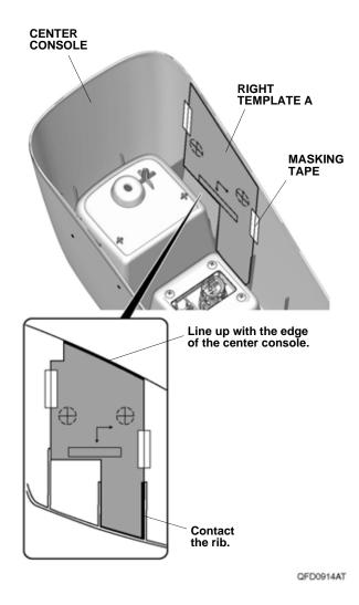
62. Using a pushpin, pierce the center of the two marks on right template A.
