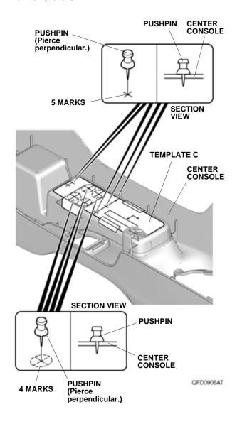
32. Using a utility knife and a felt-tip pen, mark the center console as shown.
