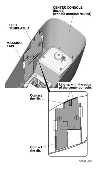
59. Using a pushpin, pierce the center of the two marks on left template A.
