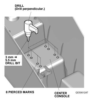
45. Using a felt-tip pen, mark the center console as shown.
