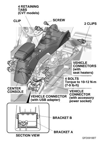
71. Install the four caps A into the center console.
