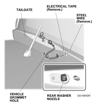
14. Connect the rear washer tube, and install the vehicle grommet.
