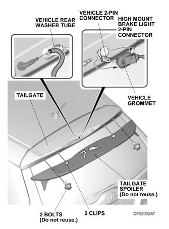
6. Remove the two grommets from the tailgate.
