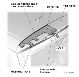
20. Use masking tape to mark the center location of the template.
