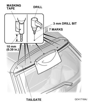
28. Attach masking tape over the seven holes as shown.
