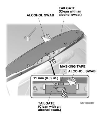
38. Use masking tape, to mark the tailgate as shown.
