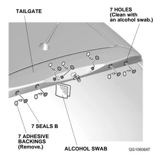
18. Remove the adhesive backings. Attach seven seals B to the tailgate as shown.
