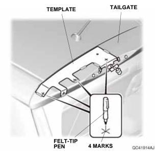
22. Turn the template over, and line up the template with the masking tape in Step 20and the tailgate as shown. Then, secure the template to the tailgate with masking tape.
