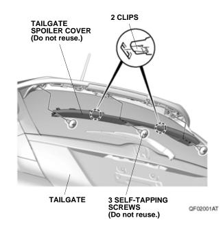
5. With the help of an assistant, remove the tailgate spoiler as shown.
