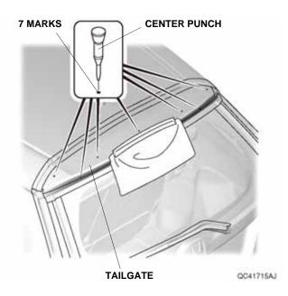
27. While wearing eye protection, drill the seven marks to 3 mm.
