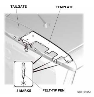
24. To prevent metal shavings from entering into the cargo area, attach masking tape to the tailgate and rear window wiper as shown.
