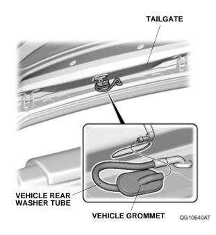
9. Close the tailgate, and remove the vehicle rear washer tube.
