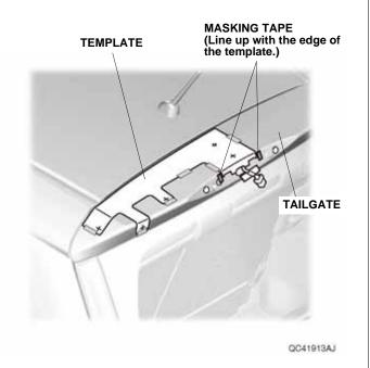
21. Using a felt-tip pen, mark the tailgate through the holes in the template. Remove the template.
