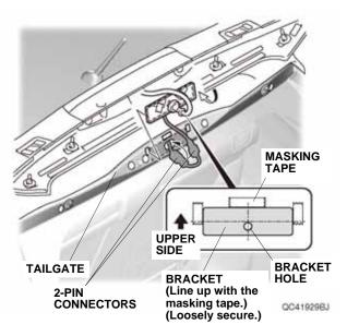
Line up the bracket with the masking tape on the tailgate as shown.
