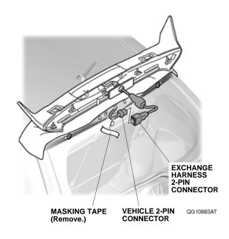
49. Peel back the adhesive backings, and tape them to the front surface of the bracket with masking tape.
