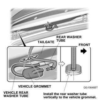
15. Close the tailgate, and connect the negative cable to the battery. Turn the ignition to ON, and test the rear washer.
