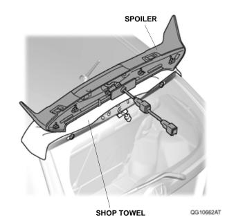
48. Remove the masking tape, and plug the vehicle 2pin connector into the exchange harness 2-pin connector.
