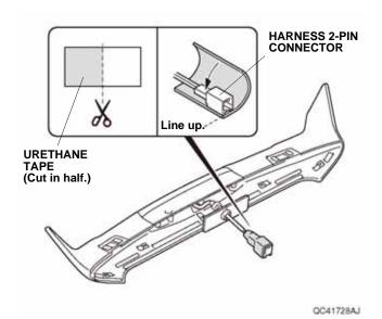
43. Plug the exchange harness 2-pin connector into the harness 2-pin connector.
