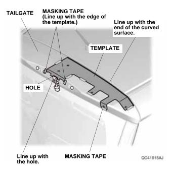
23. Using a felt-tip pen, mark the tailgate through the holes in the template. Remove the template.
