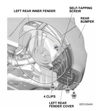
6. Remove the left rear fender cover and drain tube clip.
