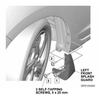
4. Turn the steering wheel fully clockwise, and repeat steps 2 and 3 to install the right front splash guard on the right side of the vehicle.
