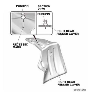
20. While wearing eye protection, drill the right rear fender cover at the pierced mark using a 3 mm drill bit first, then a 6 mm drill bit, an 8 mm drill bit, and finish using a 10 mm drill bit.
