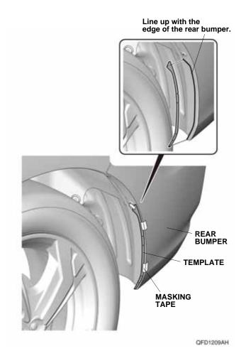
13. Using a felt-tip pen, mark the rear bumper as shown.
