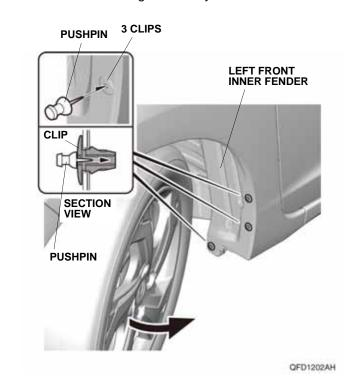
2. Using a pushpin, pierce the centers of the three clips shown on the left front inner fender.
