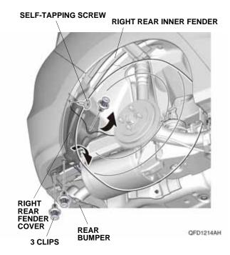
19. Locate the recessed mark. Using a pushpin, pierce the right rear fender cover at the recessed mark.
