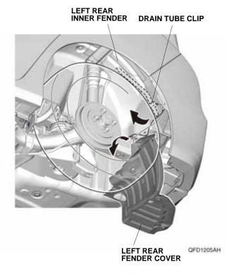
7. Locate the recessed mark. Using a pushpin, pierce the left rear fender cover at the recessed mark.
