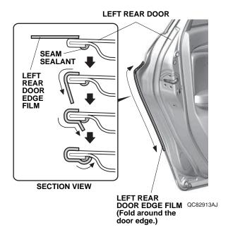
15. Using a shop towel, wipe the excess 3M protective tape application solution from the left rear door edge film. Allow the left rear door edge film to dry thoroughly.
