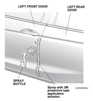
3. Open the left front door. Peel back about 50 mm (2.0 in.) of adhesive backing from the left front door edge film. Align the V-notch with the bottom of the character line on the left front door as shown.
