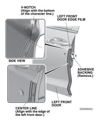
4. Align the center line on the left front door edge film with the edge of the left front door. While applying light pressure, carefully remove the adhesive backing, and attach the left front door edge film to the left front door.
