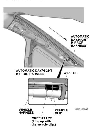
24. Secure the automatic day/night mirror harness to the vehicle harness with two wire ties.
