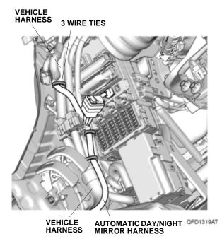
36. Route the automatic day/night mirror harness along the vehicle harness. Remove the bolt, and install the automatic day/night mirror harness ground terminal with one ground bolt.
