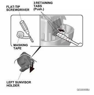
While holding down the left sunvisor holder as shown, use a flat-tip screwdriver wrapped with masking tape to remove the left sunvisor holder.
