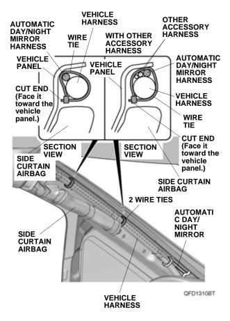
25. Route the automatic day/night mirror harness through the groove in the harness cover, and secure the harness cover to the mirror mount. Slide the harness cover behind the headliner.
