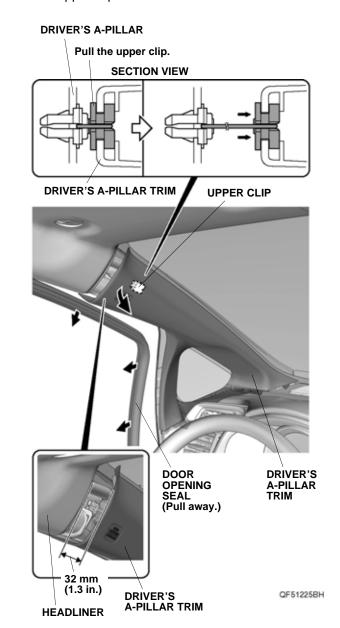
To prevent clips from falling into the body panel area, carefully insert a shop towel between the driver's A-pillar and the driver's A-pillar trim.
