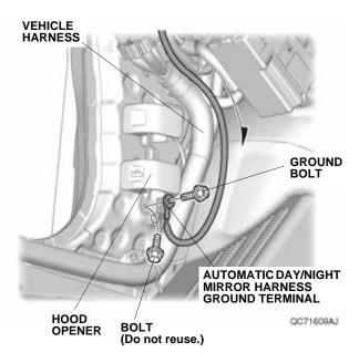
37. Secure the automatic day/night mirror harness to the vehicle harness with two wire ties.
