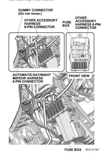
34. Plug the automatic day/night mirror harness 8-pin connector into the fuse box.
