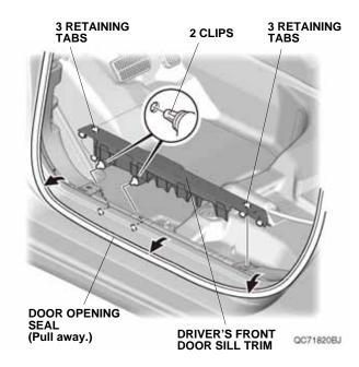
Pull away the door opening seal, and remove the driver's kick panel.
