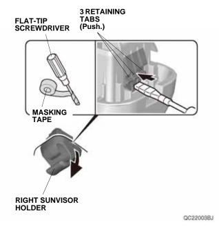
While holding down the right sunvisor holder as shown, use a flat-tip screwdriver wrapped with masking tape to remove the right sunvisor holder.
