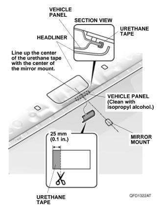
17. Using scissors, cut the urethane tape as shown, and attach one piece of urethane tape to the vehicle panel as shown. Be careful not to crease the headliner.
