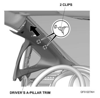
9. Remove the remaining upper clip from the driver's Apillar.
