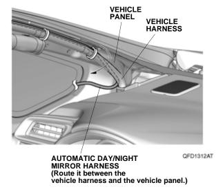
Pull away the door opening seal. Route the automatic day/night mirror harness, and tuck the automatic day/night mirror harness between the vehicle panel and the dashboard.
