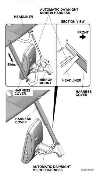
26. Route the automatic day/night mirror harness between the vehicle harness and the vehicle panel.
