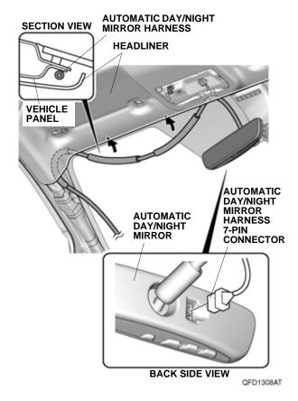
22. Gently pull back the headliner, and tuck the automatic day/night mirror harness behind the headliner. Be careful not to crease the headliner.
