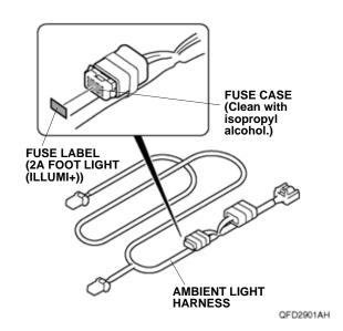
Attach the fuse label to the ambient light harness fuse case.
