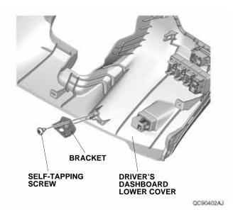
15. Install the ambient light to the bracket with one self-tapping screw.
