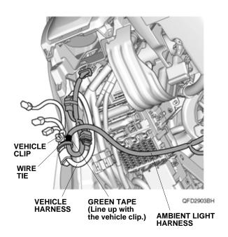
13. Route the ambient light harness as shown. Loosely secure the ambient light harness to the vehicle harness with one wire tie.
