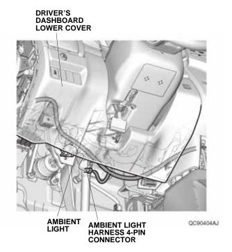
17. Secure the ambient light harness to the vehicle harness with two wire ties. If the other accessory harness is already secured to the vehicle harness, secure the ambient light harness to the other accessory harness with two wire ties. Tighten the wire tie.
