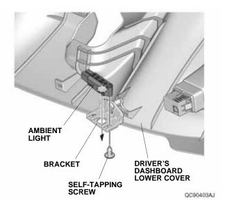
Plug the ambient light harness 4-pin connector into the ambient light, and install the driver's dashboard lower cover.
