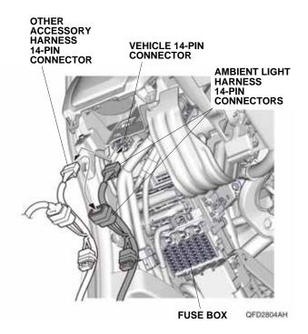
12. Line up the green tape on the ambient light harness with the vehicle clip, and secure the ambient light harness to the vehicle harness with one wire tie.
