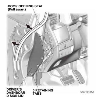
5. Remove the driver's dashboard lower cover, and unplug the vehicle connectors.
