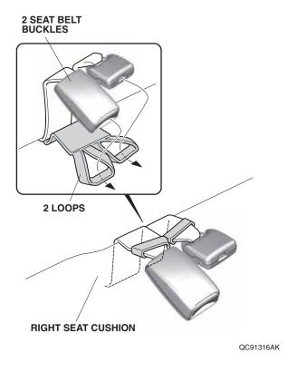
19. Lift up the right seat cushion. Secure the fasteners on the right seat cushion cover as shown.
