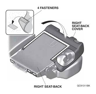
15. Lift the right seat-back. Tuck the right seat-back cover under each head restraint guide as shown.
