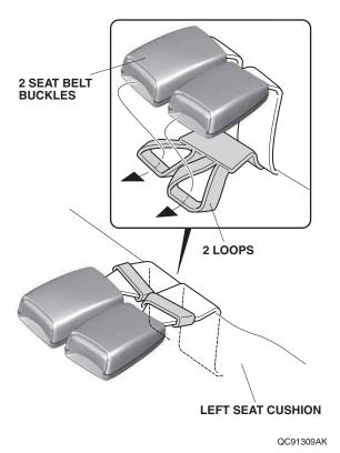
10. Lift up the left seat cushion. Secure the fasteners on the left seat cushion.
