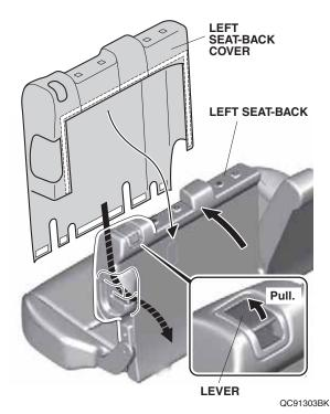
4. Lift up the left seat cushion. Secure the fastener on the left seat-back cover as shown.
