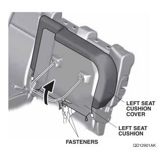
11. Secure the left seat cushion cover to the left seat cushion with two hooks and two loops, and lower the left seat cushion.
