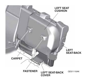
5. Lower the left seat cushion, and fold the left seatback fully forward. Pull the seat-back cover tight, and secure it to the left seat-back with the five fasteners.
