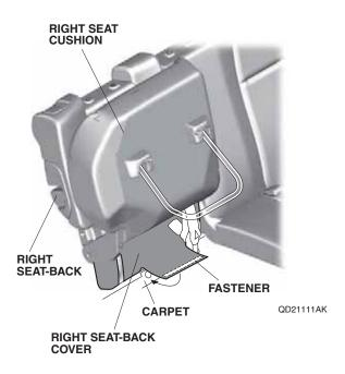
14. Lower the right seat cushion, and fold the right seatback fully forward. Pull the seat-back cover tight, and secure it to the right seat-back with the four fasteners.
