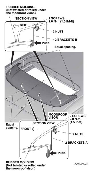
14. Tighten while applying pressure so that there is no gap between the roof panel and the brackets A and B. Torque the screws to 2.0 N·m (1.5 lb·ft).
