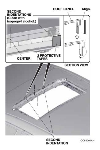
8. Remove the adhesive backings from two of the protective tapes, and attach them to the roof panel at second indentation.
