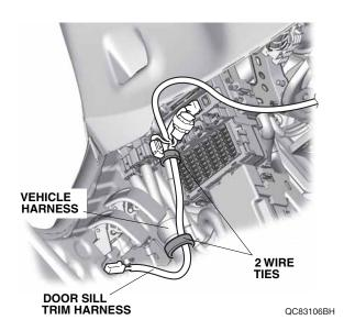
17. Route the door sill trim harness as shown. Secure the door sill trim harness to the vehicle harness with two wire ties. If other accessory harness is already secured to the vehicle harness, secure the door sill trim harness to other accessory harness with two wire ties.
