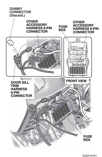
14. Plug the door sill trim harness 8-pin connector into the fuse box.
