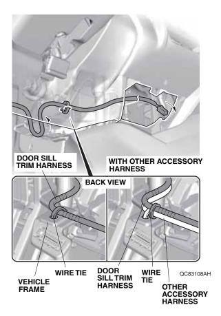
Secure the door sill trim harness to the vehicle harness with one wire tie.
