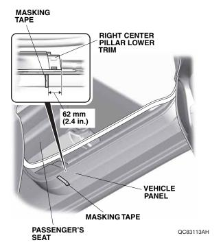
25. Align the edge of the right front illuminated door sill trim with the edge of the masking tape.
