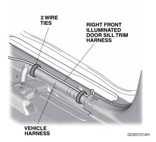
51. Using a utility knife, cut the driver's front door sill trim in the area shown.
