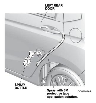
10. Open the left rear door. Peel back about 50 mm (2.0 in.) of adhesive backing from the left rear door edge film. Align the V-notch 40 mm (1.6 in.) above the character line on the upper part of the left rear door as shown.
