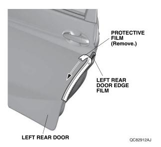
14. Starting from the center and working outward, use your fingers to fold the left rear door edge film around the edge of the left rear door as shown. Move your fingers in one direction only. Attach the left rear door edge film over the seam sealant. Do not trim or damage the seam sealant.
