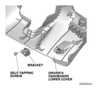
14. Install the ambient light to the bracket with one self-tapping screw.
