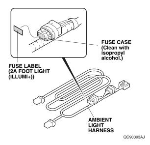
9. Attach the fuse label to the ambient light harness fuse case.
