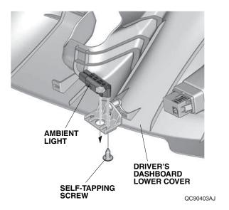
15. Plug the ambient light harness 4-pin connector into the ambient light, and reinstall the driver's dashboard lower cover.
