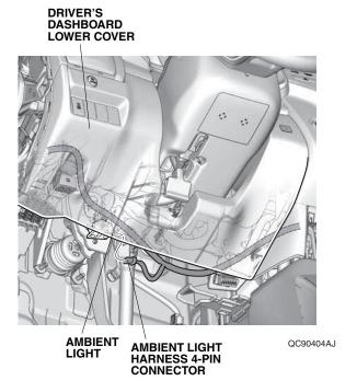
16. Secure the ambient light harness to the vehicle harness with two wire ties. If other accessory harness is already secured to the vehicle harness, secure the ambient light harness to other accessory harness with two wire ties. Tighten the wire tie.
