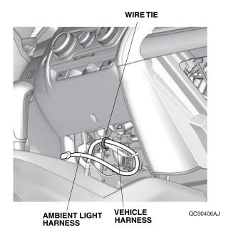
18. Route the ambient light harness as shown. Secure the ambient light harness to the vehicle harness with three wire ties.
