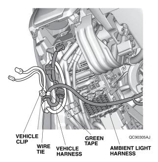
12. Route the ambient light harness as shown. Then loosely secure the ambient light harness to the vehicle harness with one wire tie.
