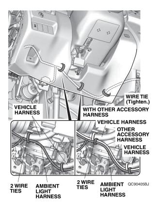
17. Secure the ambient light harness to the vehicle harness with one wire tie.
