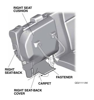
14. Lower the right seat cushion, and fold the right seatback fully forward. Pull the seat-back cover tight, and secure it to the right seat-back with the four fasteners.
