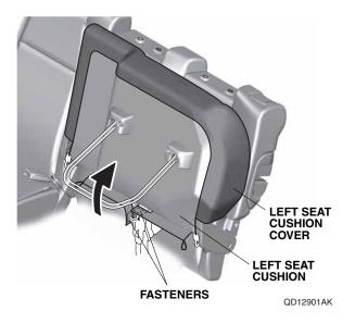
11. Secure the left seat cushion cover to the left seat cushion with two hooks and two loops, and lower the left seat cushion.
