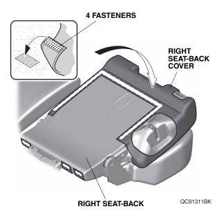
15. Lift the right seat-back. Tuck the right seat-back cover under each head restraint guide as shown.
