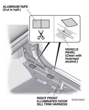
49. Using scissors, cut one aluminum tape in half. Secure the right front illuminated door sill trim harness to the vehicle panel with aluminum tape.
