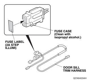
Attach the fuse label to the door sill trim harness fuse case.
