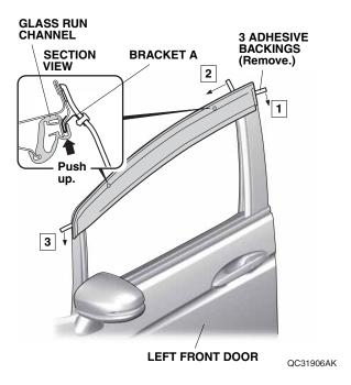
9. Using a soft towel, press and hold the left front door visor against the door sash for 30 seconds.
