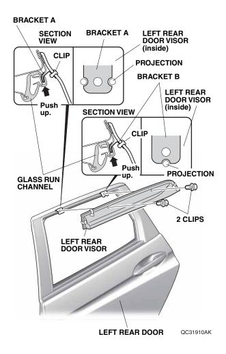
Adjust the left rear door visor to the position as shown.
