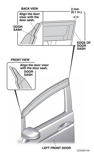
8. While applying light pressure against the left front door visor, carefully remove the adhesive backings in the order shown. Use your finger to push up each bracket so there is no gap between the bracket and the door sash.
