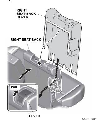
13. Lift up the right seat cushion. Secure the fastener on the right seat-back cover as shown.
