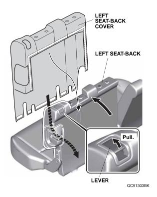
4. Lift up the left seat cushion. Secure the fastener on the left seat-back cover as shown.
