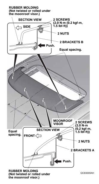
Tighten while applying pressure so that there is no gap between the roof panel and the brackets A and B. Torque the screws to 2.0 N·m (0.2 kgf·m, 1.5 lbf·ft).
