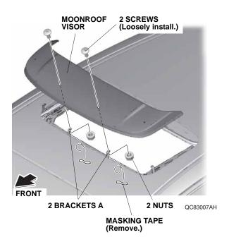
12. Loosely install the moonroof visor to the brackets B with two screws and two nuts. Remove the masking tape from the brackets.
