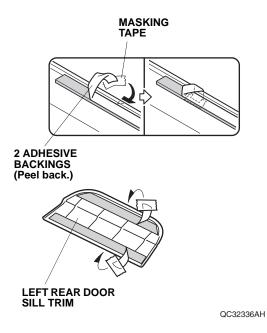
58. Using an alcohol swab, thoroughly clean the area where the left rear door sill trim will attach.
