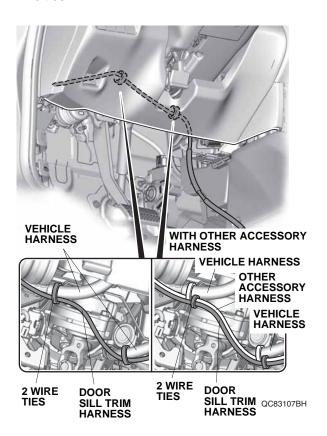
18. Route the door sill trim harness as shown. Secure the door sill trim harness to the vehicle frame with one wire tie. If other accessory harness is already secured to the vehicle frame, secure the door sill trim harness to other accessory harness with one wire tie.
