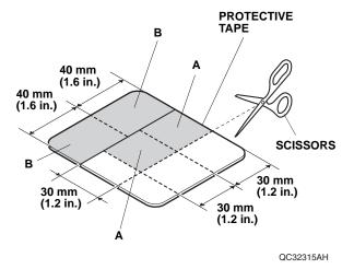
24. Attach masking tape to the vehicle panel at the measurement shown.
