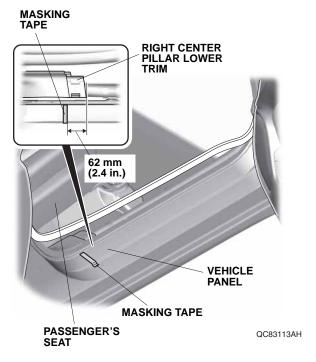
25. Align the edge of the right front illuminated door sill trim with the edge of the masking tape.
