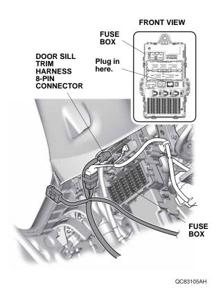
15. Attach the door sill trim harness fuse case to the vehicle connector.
