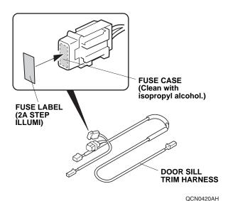
1. Attach the fuse label to the door sill trim harness fuse case.
