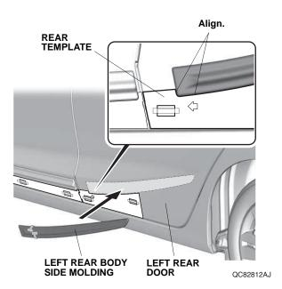
15. Press on the left rear body side molding lightly with the palm of your hand while removing about 50 to 100 mm (2.0 to 4.0 in.) of the adhesive backings at a time.
