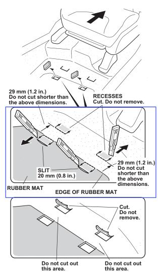
Locate the two recesses in the carpet. Using a utility knife, slit the carpet at the front of the recess in the direction shown. Be careful not to cut out the piece between the recess and the rubber mat, otherwise the entire floor carpet must be replaced.
