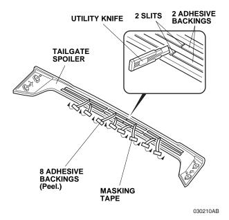
18. Attach a piece of masking tape to the end of the adhesive backings as shown. Peel back the adhesive backings partway and temporarily attach them to the front surface of the tailgate spoiler.
