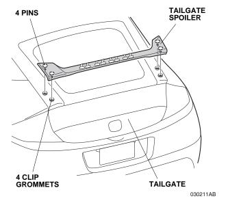
20. Adjust the position of the tailgate spoiler as shown.
