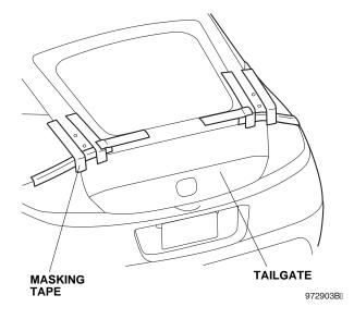
11. While wearing eye protection, drill the four centerpunched marks on the tailgate with an 8.5 mm hole cutter.
