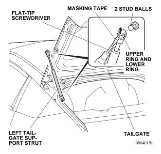
3. Install the left tailgate support strut to two stud balls on the tailgate.
