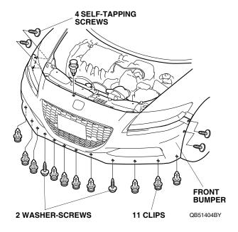
Release two retaining tabs on each side of the bumper.
