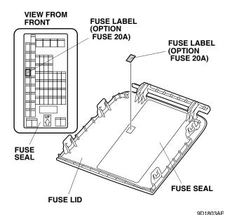
48. Using an isopropyl alcohol on a shop towel, thoroughly clean the fuse lid where the blank fuse label will attach. Attach the fuse label to the fuse seal of on the fuse lid as shown.
