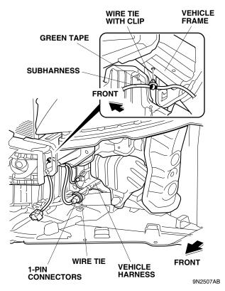
Secure the 1-pin connectors to the vehicle harness with one wire tie. 34. With the help of an assistant, bring the front bumper close to the vehicle. Plug the subharness 4-pin connector into the fog light harness 4-pin connector and reinstall the front bumper.
