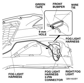
24. Align the green tape on the fog light harness to the 9 mm hole and secure the fog light harness to the front bumper with one wire tie.
