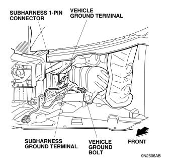
32. Locate the green tape on the subharness. Install the wire tie with clip to subharness at the green tape. Insert the wire tie with clip into the hole in the vehicle frame.
