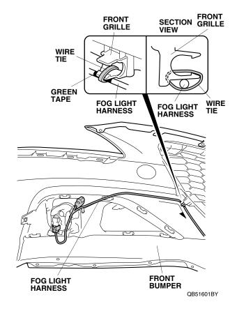
23. Route the fog light harness, and plug the fog light harness 2-pin connector into the right fog light.
