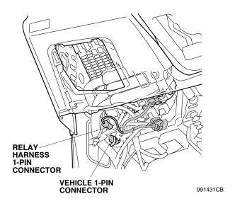
Remove lower hood opener bolt, and secure the relay bracket to the vehicle panel with the hood opener bolt.
