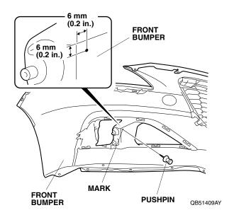
13. While wearing eye protection, drill the pierced mark in the front bumper with a 3 mm drill bit.
