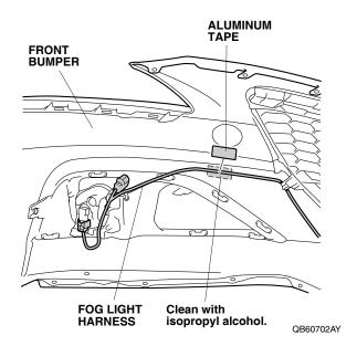
27. Secure the fog light harness to the front bumper with one aluminum tape.
