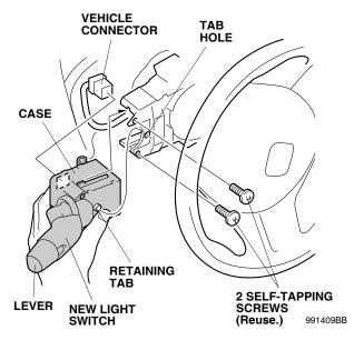
45. Plug the vehicle connector to the new light switch. Make sure the vehicle harness is not being stretched.
