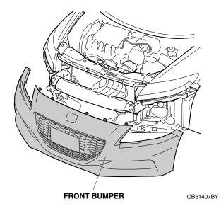
11. Remove the left cover from the front bumper (one clip and eight retaining tabs).
