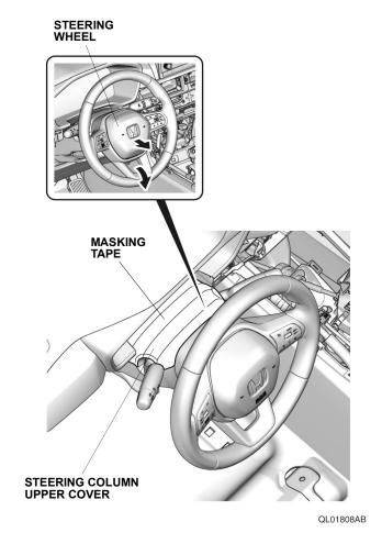
11. Attach masking tape to protect the vehicle.
