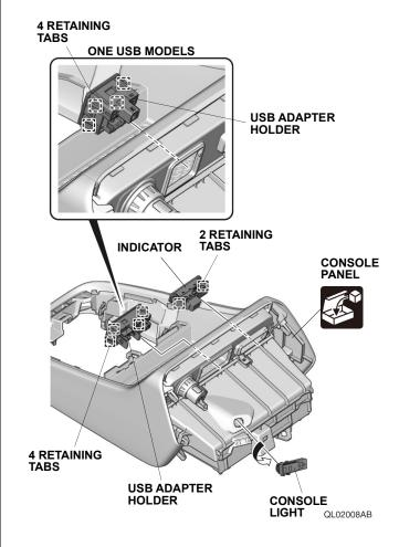
28. Install the USB adapter holder, indicator, and console light.
