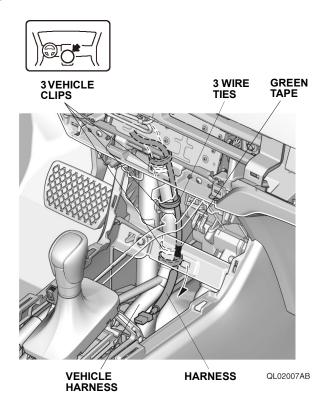
27. Remove the USB adapter holder, indicator, and console light.
