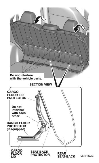
12. Check that all parts are installed properly.
