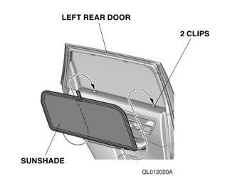
2. Install the top of the sunshade into the clips, by pulling straight down on the tab.
