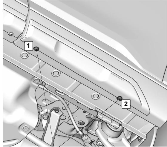
2 WASHER-SCREWS (Tighten.)
