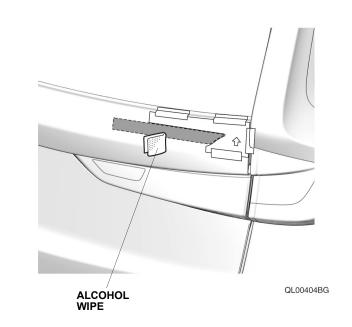
3. Temporarily attach the adhesive backing.
