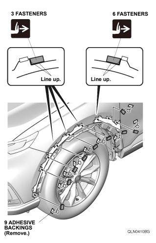
11. Secure the fasteners.
