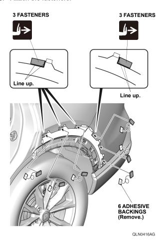
24. Secure the fasteners.
