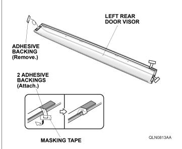
17. Remove the adhesive backing.
