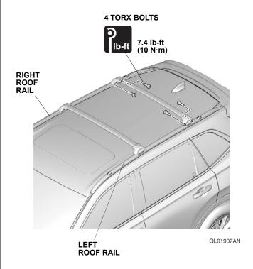
7. Check that all parts are installed properly.
