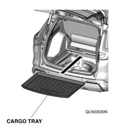
2. Reinstall the cargo floor board into the upper position over the cargo tray.
