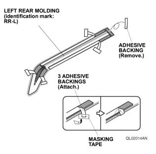
17. Remove the adhesive backing.
