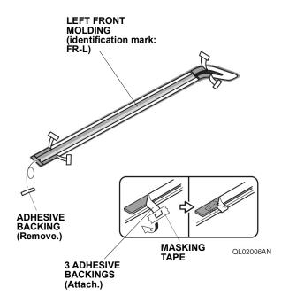
6. Remove the adhesive backing.
