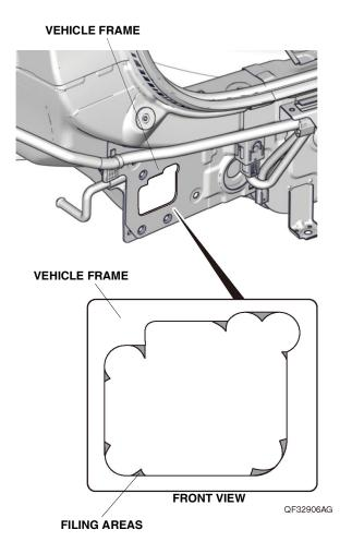
43. Apply touch-up paint to the edge of the hole. Allow the touch-up paint to dry thoroughly.
