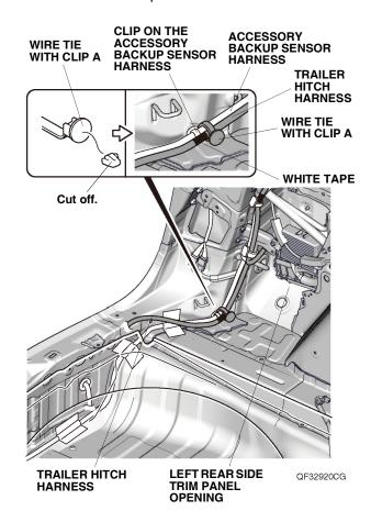
71. Line up the white tape on the trailer hitch harness with the clip on the accessory backup sensor harness, and secure the trailer hitch harness to the accessory backup sensor harness with one wire tie with clip A. Go to step 73.
