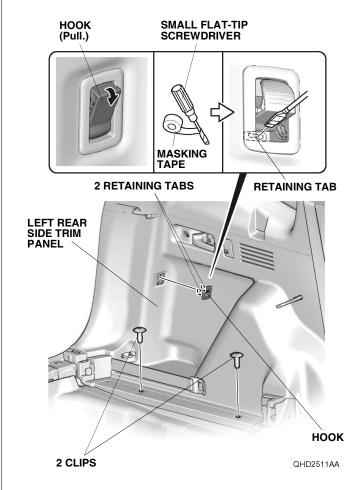
Apply masking tape to the left rear side trim panel as shown.
