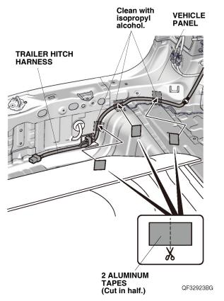
76. Using scissors, cut the two pieces of aluminum tape in half, and secure the trailer hitch harness to the vehicle panel with three halves of aluminum tape as shown.
