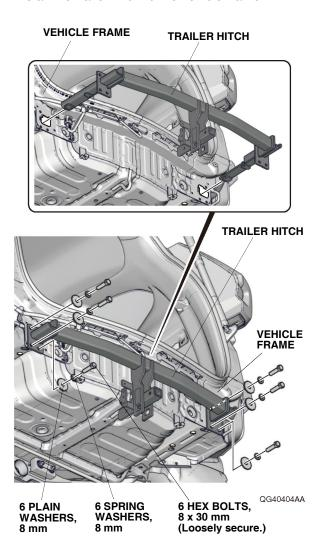
48. Loosely secure the trailer hitch to the vehicle frame with six 8 mm plain washers, six 8 mm spring washers, and six 8 x 30 mm hex bolts.
