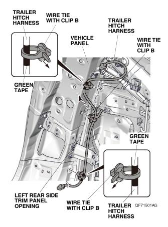
67. Secure the trailer hitch harness to the vehicle panel with one wire tie with clip B.
