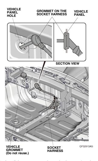
57. Install the grommet on the socket harness into the vehicle panel hole.
