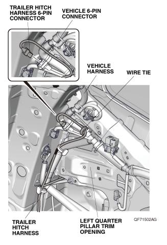
Secure the trailer hitch harness to the vehicle harness with one wire tie. If the vehicle is equipped with the accessory backup sensors, continue with step 70; otherwise, go to step 72.
