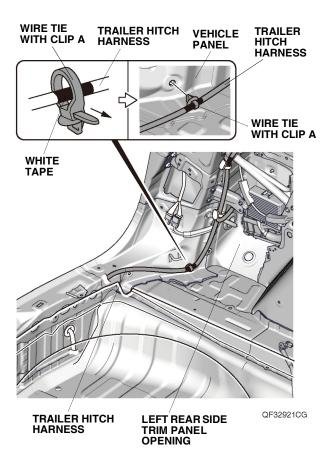
73. Peel back the floor carpet, then route the trailer hitch harness as shown.
