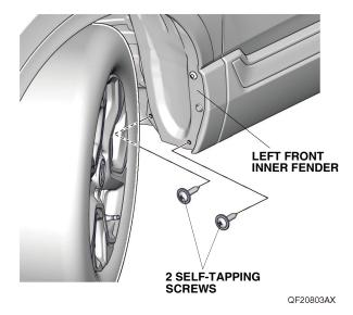
Loosely secure the left front splash guard on the left front inner fender with one 5 x 25 mm self-tapping screw and two self-tapping screws removed in step 3.
