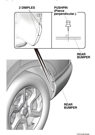
8. Thread the 5 x 25 mm self-tapping screw into the pierced dimple. Remove the self-tapping screw. Repeat for the other dimple.
