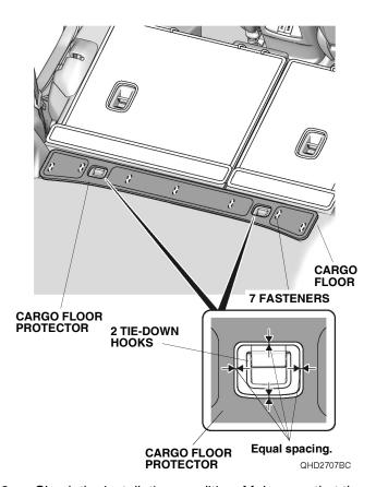
Check the installation condition. Make sure that the protectors do not interfere with the vehicle parts while moving the left and right rear seat-backs back and forth.
