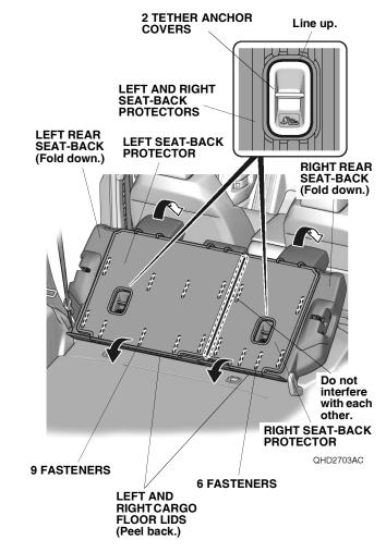
4. Remove the protective clothes from the left and right cargo floor lid protectors.
