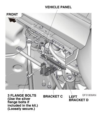
26. With the help of an assistant, loosely secure the left running board to bracket A, bracket B, bracket C, and left bracket D with 13 flange bolts. NOTE: If there are black and silver flange bolts in the kit, use six black flange bolts and seven silver flange
