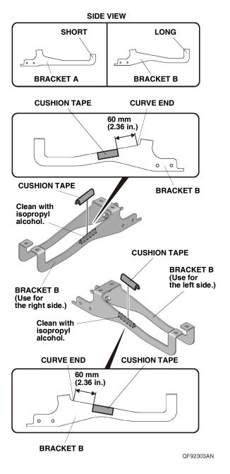
17. Attach one cushion tape to each bracket B as shown. Make sure to attach the cushion tapes in the correct position and orientation.
